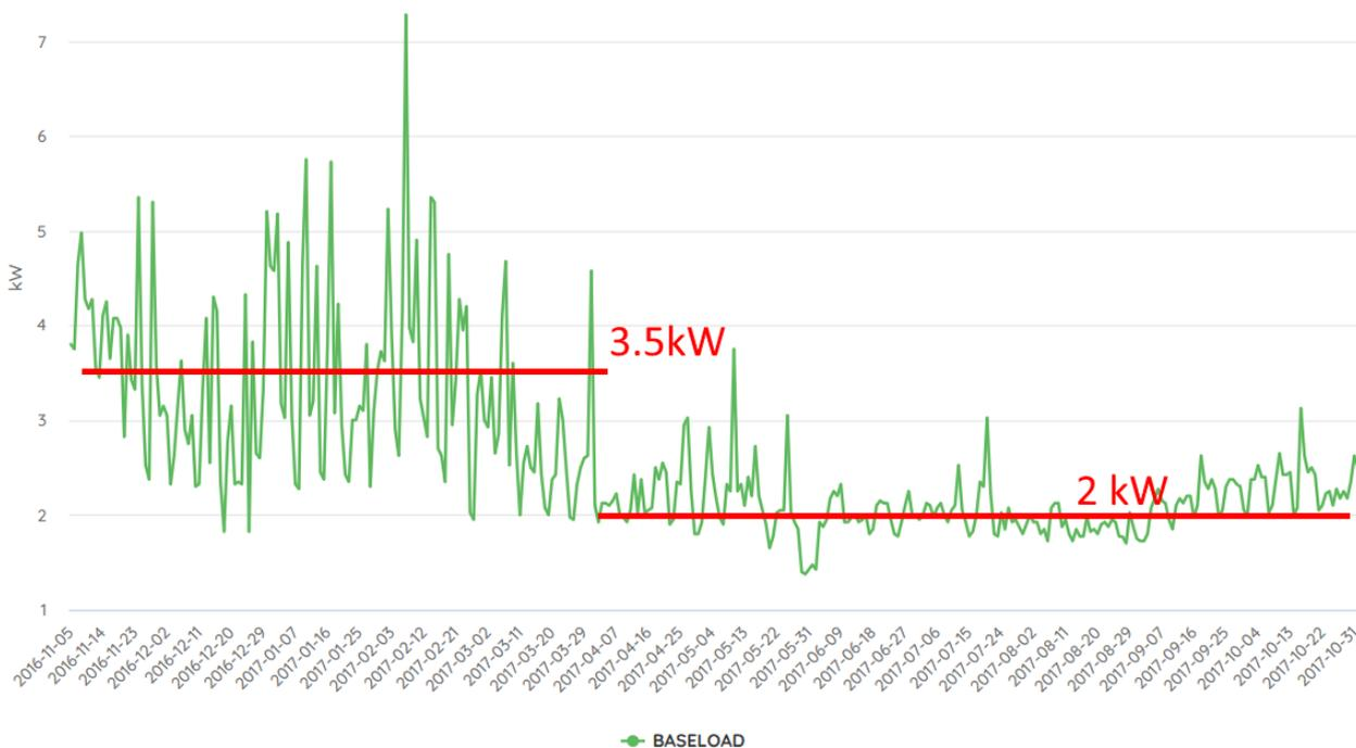
The baseload dropped 1.5 kW from 3.5 kW to 2 kW. This is about a 13,000 kWh and £1,600 annual reduction in electricity consumption. This one change represented as 23% reduction in the school's annual electricity consumption.
